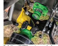
Quik Knect™ PTO receivers make for easy PTO connections in seconds.
