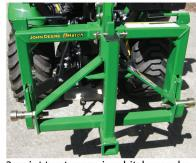
3-point tractor receiver hitches make moving trailers easy.
